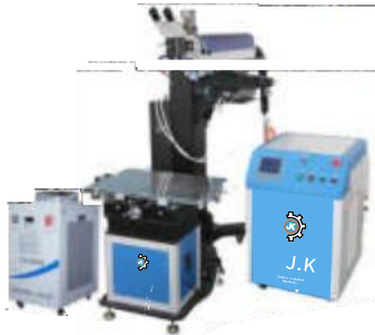
LASER WELDING (Pg. No. 11)
